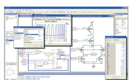
Tanner S-Edit Schematic capture design and simulation cockpit shows schematics, simulation waveforms, model parameters, and simulation settings; the tool is easy to use and has the power to handle complex mixed-signal IC design capture.
